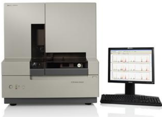
Figure 4.2 The ABI genetic analyzer 3130. This is a four capillary electrophoresis sequencing platform. It uses the 96-well micro PCR plates.
