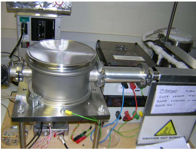
Fig. 3.4: The vacuum chamber of the Poling Rig
