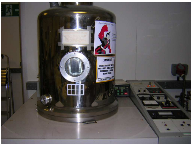
Fig. 3.2: The Edwards E480 thermal evaporator
