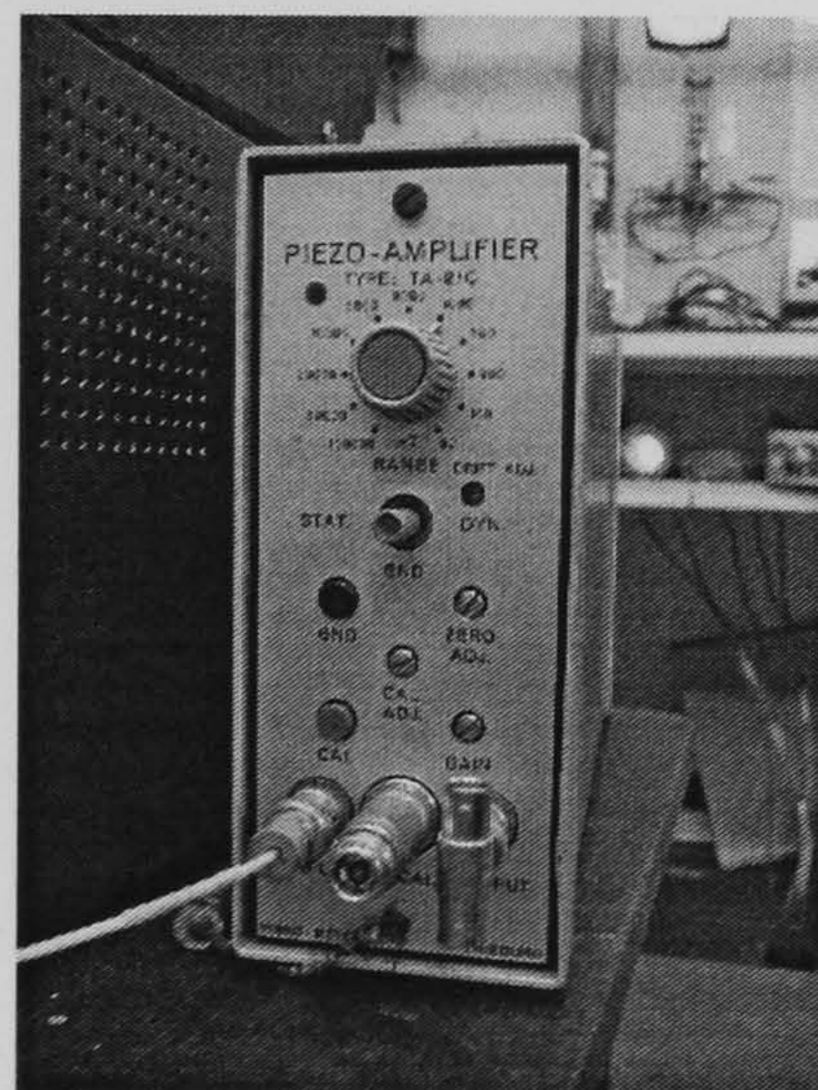
Figure 5.25 Charge amplifiers for pressure transducer
