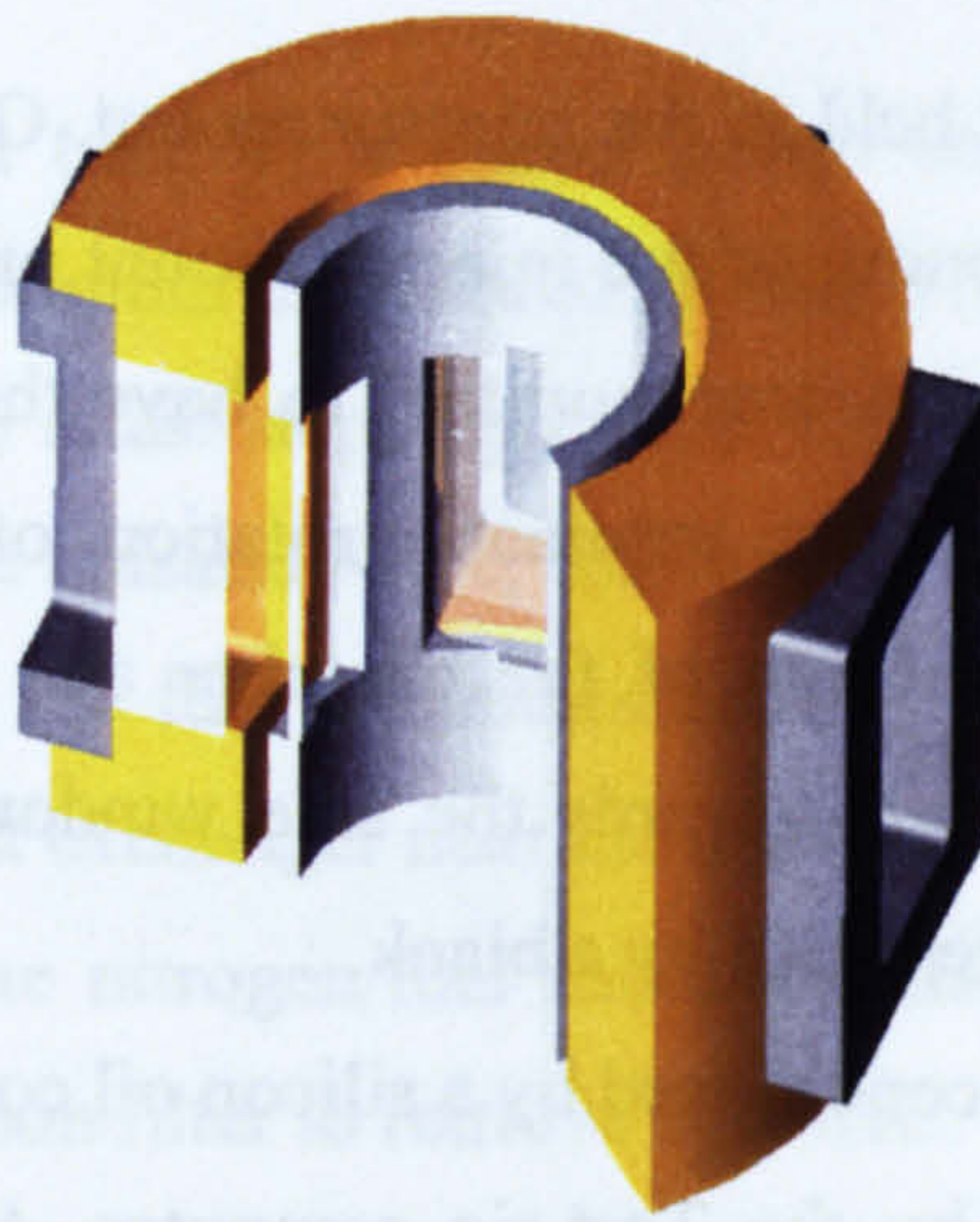
Figure 4-2: Cutaway section of the Mie/LIF Pressure vessel - inner/outer cylinder, windows and window holders
