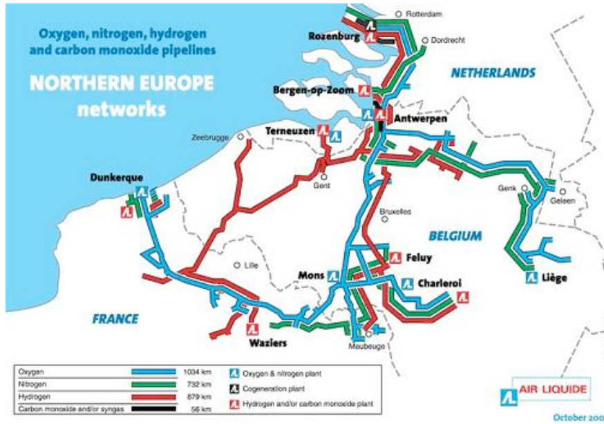
Figure A.9. Gas distribution network of Air Liquide, adopted from Air Liquide (2009).
