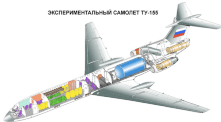
Figure 1.12. The hydrogen fueled Tupolev TU-155 aircraft, adopted from Kaminski-Morrow (2009).
