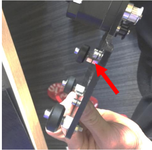
Figure 3.2-1: Original rail guides for x axis gantry
