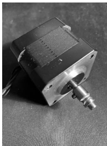
Figure 2.7-2: Extruder stepper motor with 92t hobbed gear
