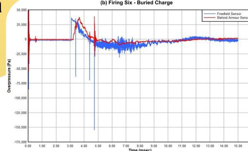
Results of experimental work looking at the effect of changing the location of a charge when (a) the charge was placed in free field and (b) when the charge was buried 10cm underground.
