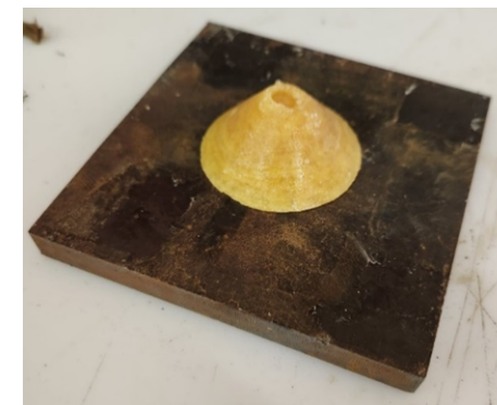
Cast TNT 90 deg cone (30g)
