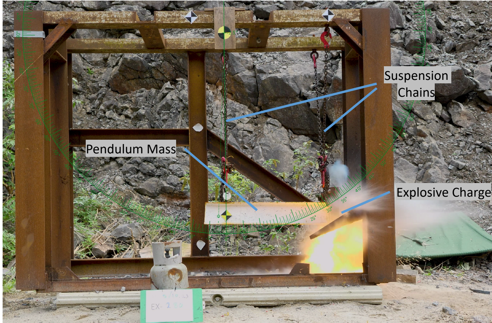
Poladyn charge. Note the sacrificial anvil between the charge and the pendulum mass
