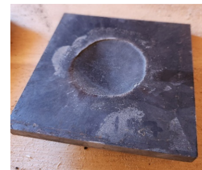
Typical "dent" from plastic explosive
