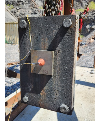
Poladyn charge. Note the sacrificial anvil between the charge and the pendulum mass
