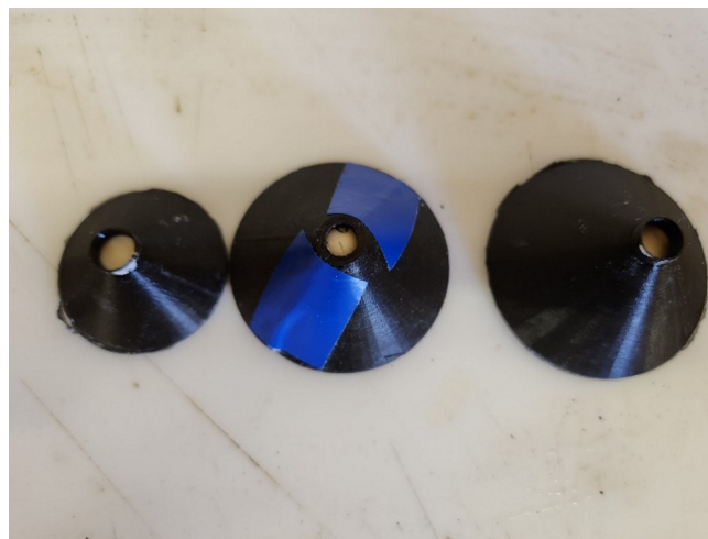
PE4 90 deg. Cones in sacrificial moulds (10g, 20g, 30g)
