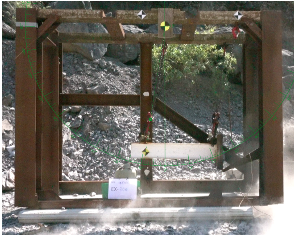
(b) Fig. 3. (a) The 86kg pendulum mass has replaceable anvils and each charge has one or more sacrificial steel anvil plates to protect the pendulum mass from damage (b) The MBP frame and light mass being swung by a 30g charge of plastic explosive. “Tracker” software allows accurate measurement of the angle of rotation from recorded video.
