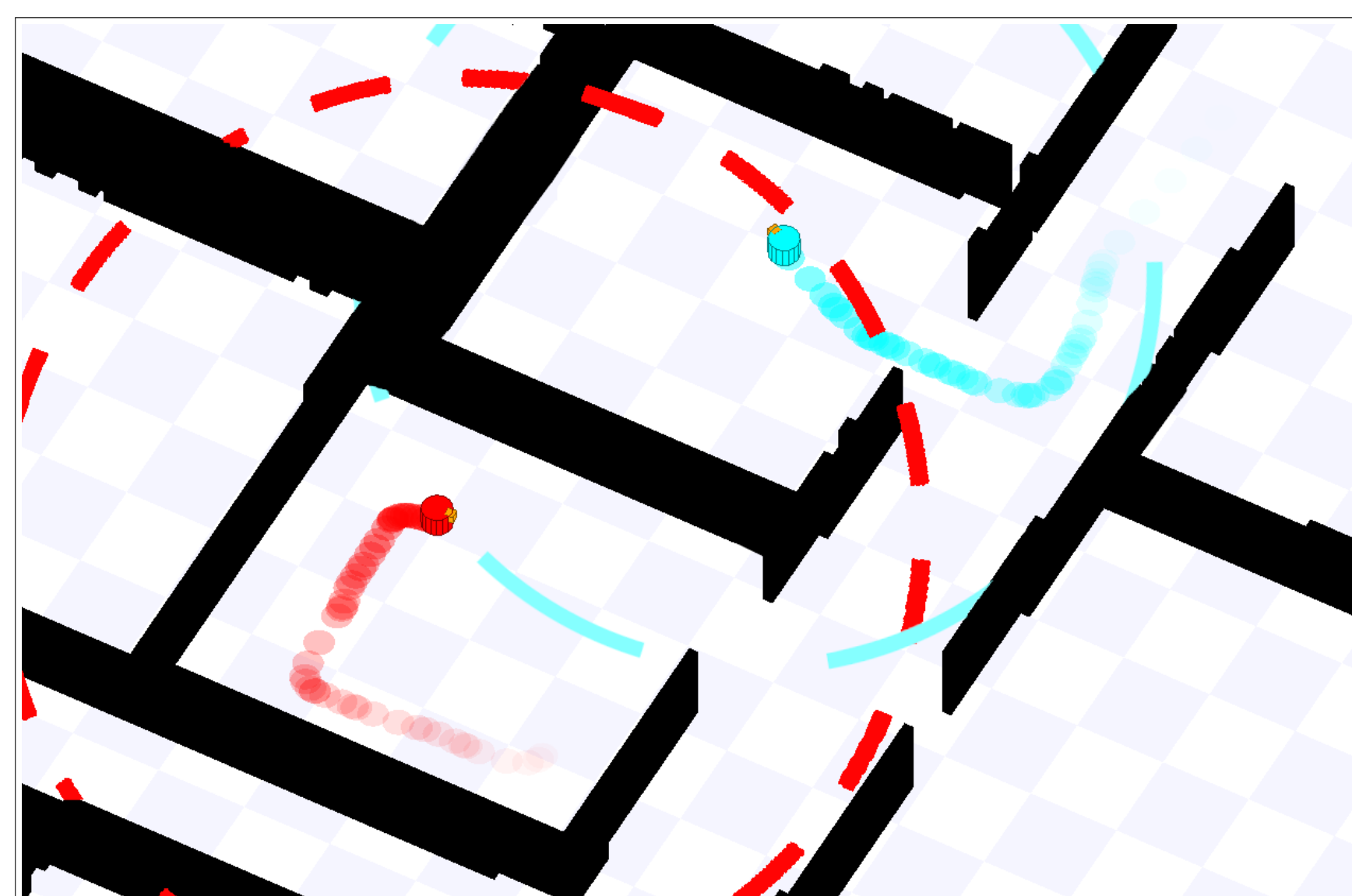
Figure 2: Communication radii of two robot agents patrolling.
