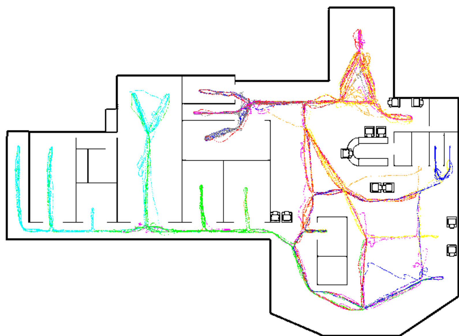
Figure 1: Trajectory plot of a system of eight robots executing the SEBS patrol algorithm for over an hour, with each unique color representing a single robot and its patrol route.
