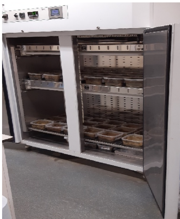
Figure 3.1. Experimental setup for biostimulation treatment of hydrocarbon contaminated acidified wetland soil.
