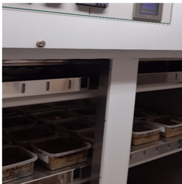
Figure 5.1. Experimental setup for optimised combined biostimulation and bioaugmentation treatment of hydrocarbon contaminated acidified wetland soil.
