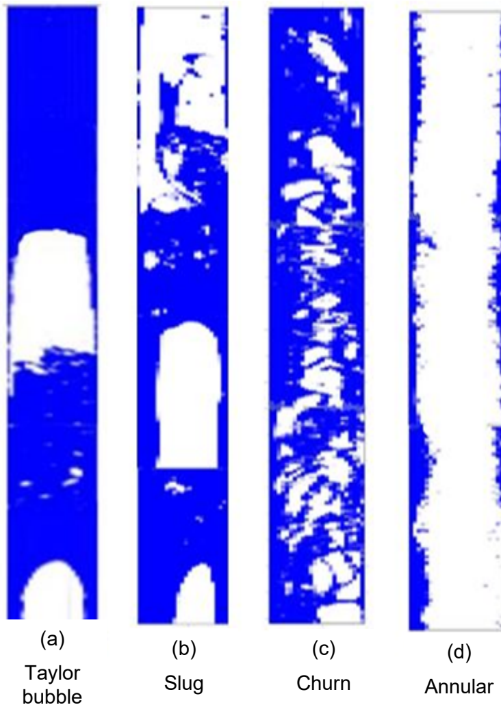
Figure 4-4 Axial slice images of the two-phase flow regimes in vertical section at superficial gas and liquid velocities of (a) 0.14 m/s and 0.043 m/s (b) 1.36 m/s and 0.043 m/s (c) 2.73 m/s and 0.43 m/s and (d) 10.91 m/s and 0.043 m/s.
