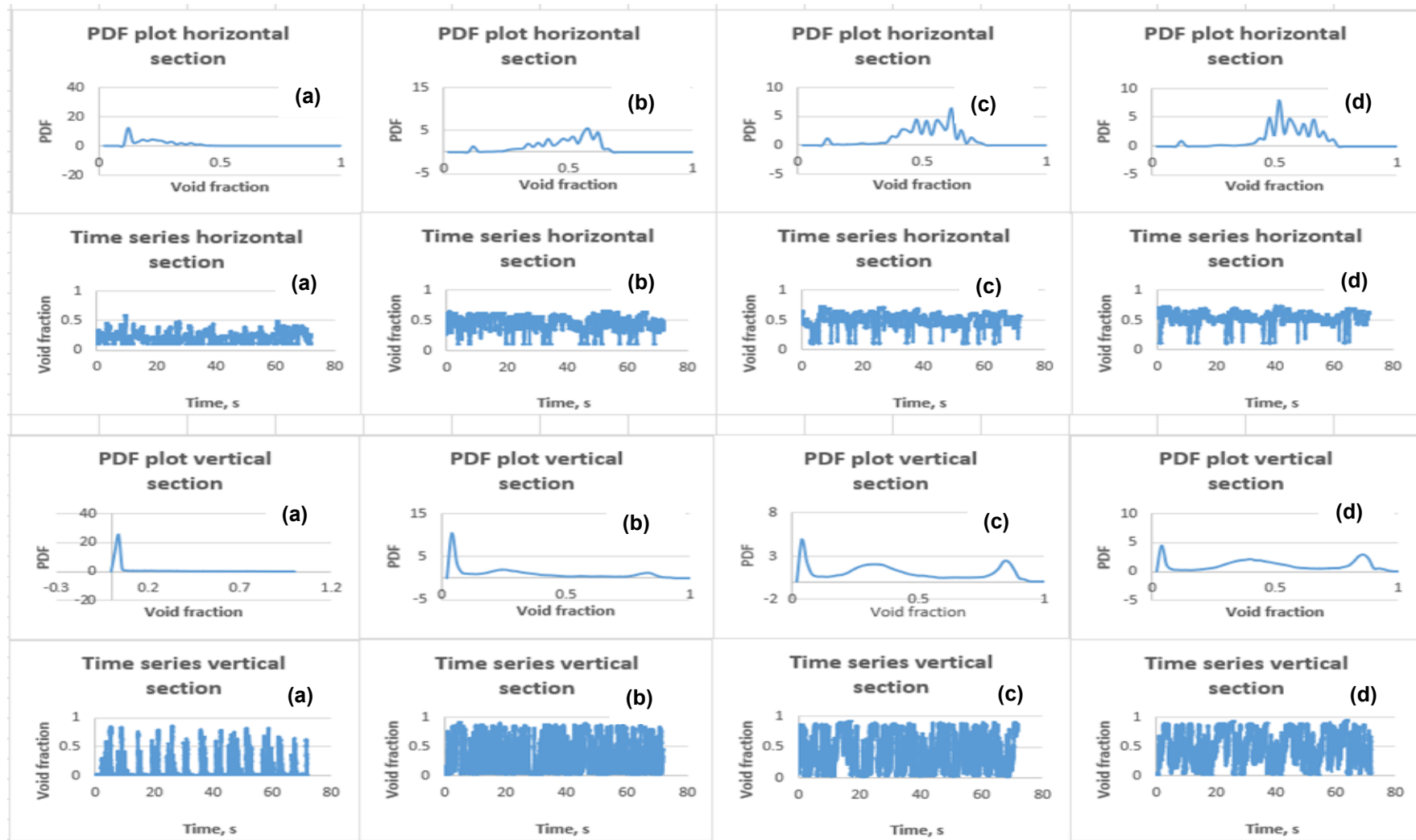
Figure 4-14 PDF and time series plots of horizontal and vertical flows for 100D with superficial liquid velocity of 0.086 m/s and superficial gas velocities of (a) 0.14 m/s (b) 0.55 m/s (c) 0.95 m/s and (d) 1.36 m/s.
