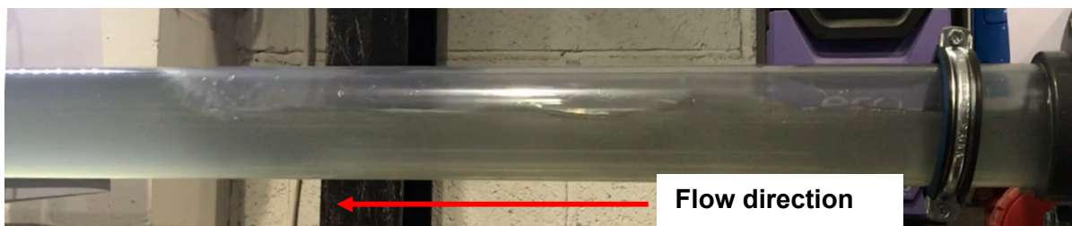
Figure 4-2 Picture of unstable wavy-slug (UWS) flow regime for superficial velocities of 0.55 m/s and 0.043 m/s for gas and liquid respectively with 100D gas injection point.
