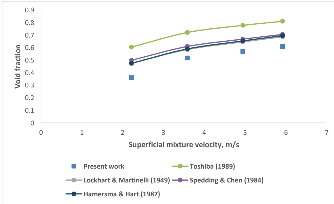
Figure 4-24 Plot of the relationship between void fraction and mixture superficial velocity to compare void fraction correlations used in conventional horizontal pipe with that of present work for flows with U_{sl} = 0.43 m/s and U_{sg} = 1.36 - 5.45 m/s.
