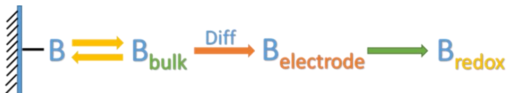
Figure 3-14 Scheme of the desorbing electrochemical process with an absorbed molecule B.
