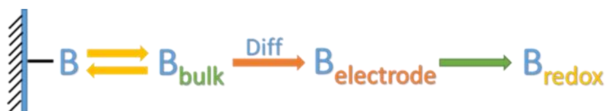
Figure 4-16 A complete electrochemical process of a substrate molecule B
