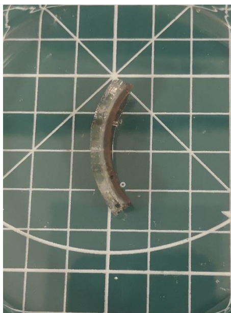
Figure 6-5 The three-layer structure of polymer reactor PRS
