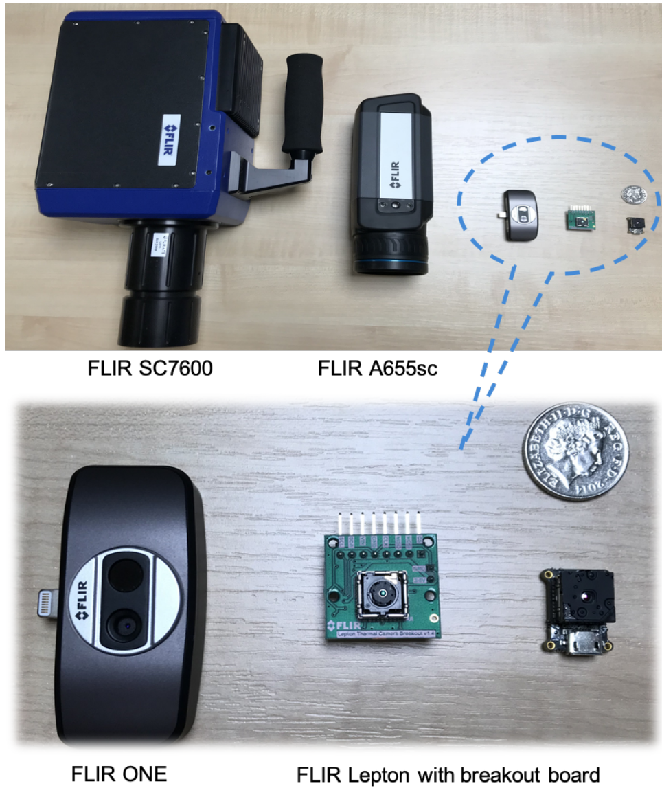
Figure 3-3 Comparison of the FLIR lepton with FLIR ONE, SC7600 and A655sc
