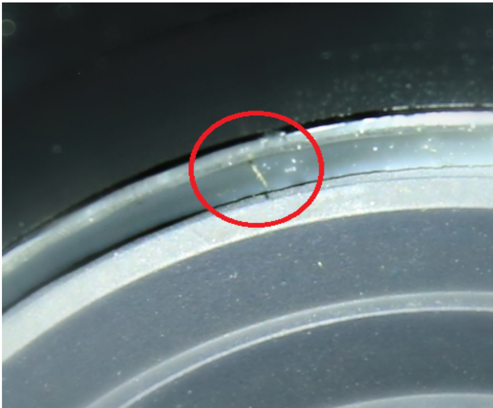
Figure 4-5 A snapshot of the observed 'v' shape feature (red circled) shown in Zone 2.
