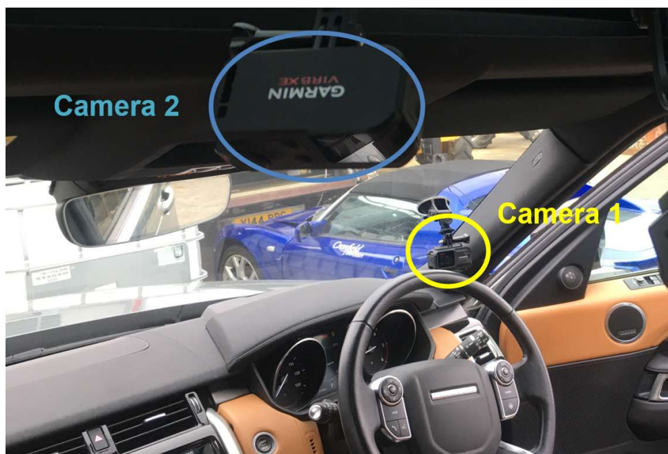
Figure 6-4 A illustration of the two cameras inside the vehicle
