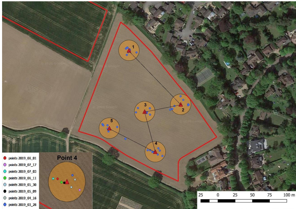
Figure 3-2 Sample collection from Sawyers_3 field creating a W shape across the field with the total samples (blue) from different dates. The centroid (red) is calculated by the repeated blue dots assigned in each point (red). This centroid provides the area with a radius of 15 m creating plots (orange) to extract the SAR polarisations for the individual points in the field. The field is buffered 10 m to reduce the effect of the field boundaries in SAR.
