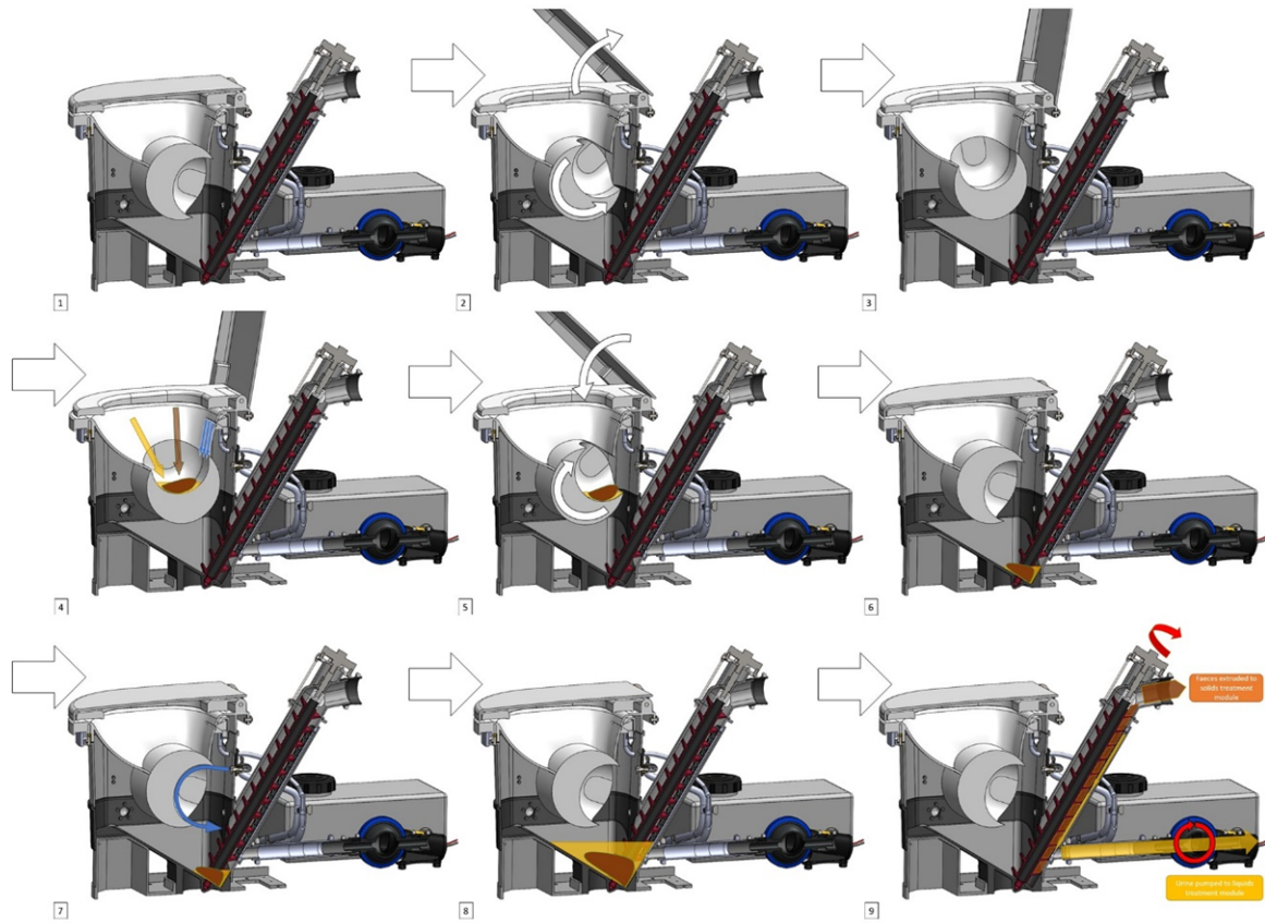
Figure 29 Waste Evacuation Steps in User-Interfacing Module
