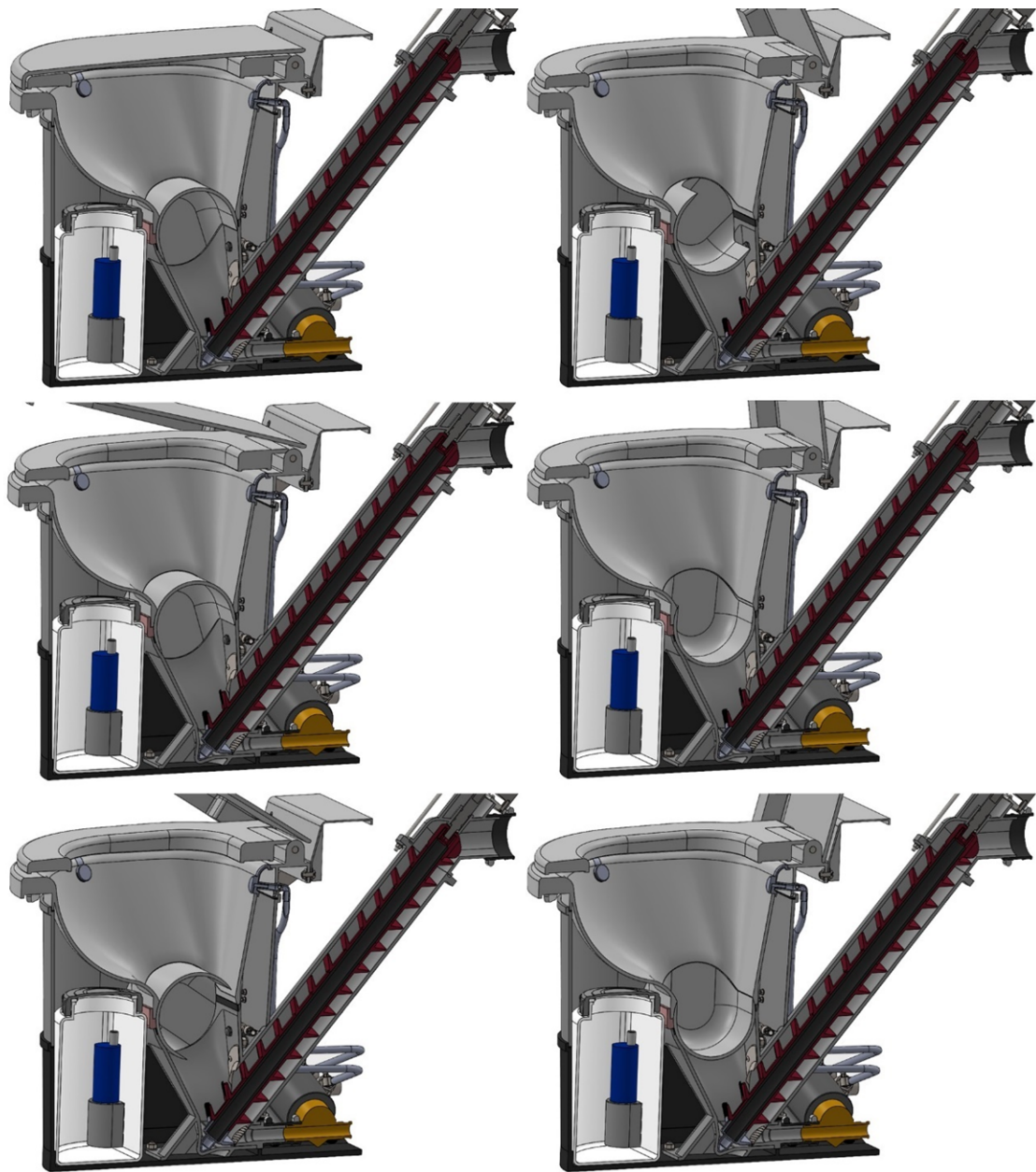
Figure 32 Proposed user-interfacing module - lid motion sequence with cross-section view
