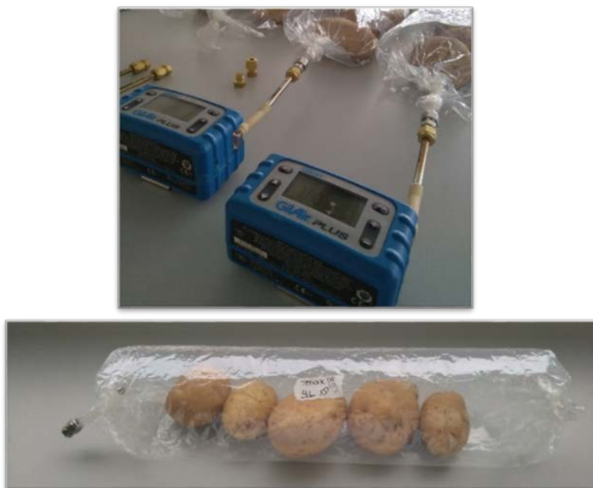
Figure 2-6 Potato tubers incubation in nalophan bags and air sampling using a TD tube connected to the Gil air plus Air Pump (Sensydine, USA).
