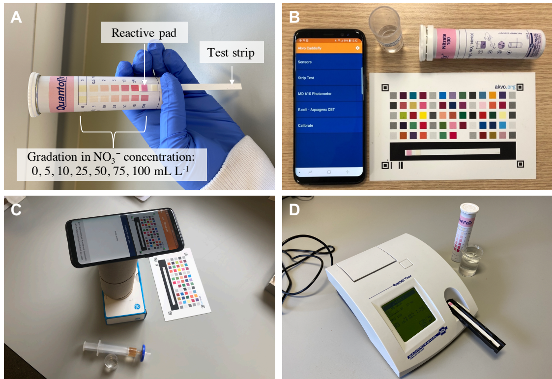
Figure 3-1. Semi-quantitative paper test strips and two types of reflectometers, i.e. devices that quantify colour. Discerning colours of the reactive pad raises issues in terms of inter-rater agreement and replicability due to gradation range and the semi-quantitative nature of test strips (A). Akvo Caddisfly set-up during the laboratory works (B), the app together with the calibration card and nitrate-
