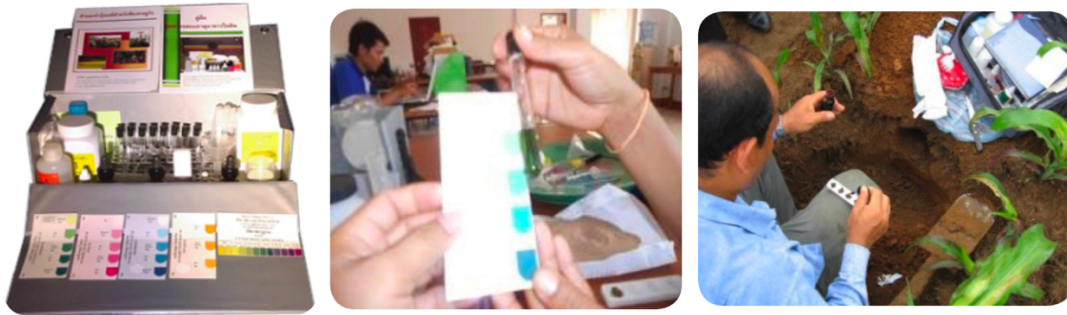
Figure 1-1. In-field test kits employed in soil fertility assessment in South East Asia. The kits consist of qualitative and semi-quantitative colorimetric charts. The deeper the colour, the higher the quantity of the measured nutrient (from Nyi et al., 2017).
