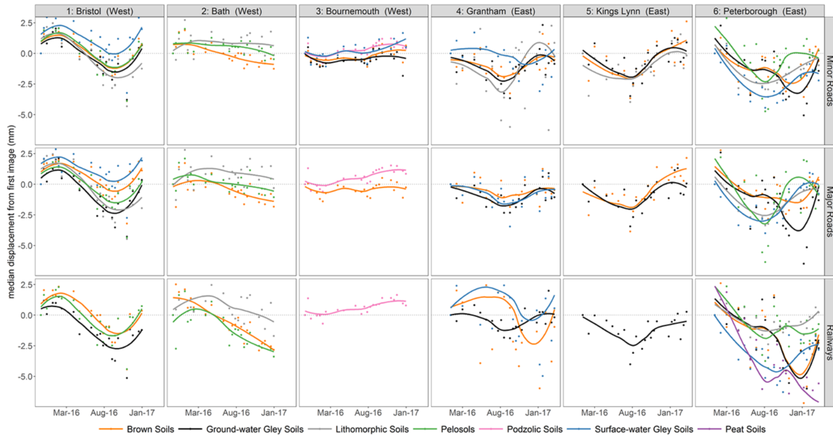
Figure 5-4: Trends in vertical movement (mm) by major soil group and infrastructure type. Points show median value for all PSI points on an infrastructure type and major soil group. Solid line show a loess-smoothed trend through the plotted medians. Dashed lines identify 1st January. To ensure validity, classes with less than 100 PSI points have been removed from this plot (Table 5-5)
