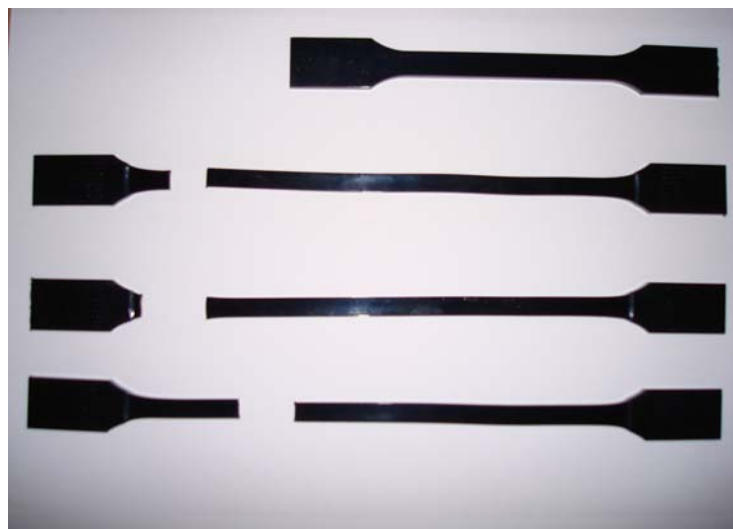
Figure 4.6 Failed Test Pieces tested at 50mm/min
