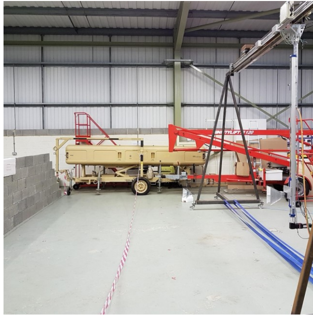
Figure 4-21 – Photograph of the measurement setup. One antenna is placed on a polystyrene plinth facing towards the centre of the wall. The other antenna traverses a linear trajectory at a constant height.
