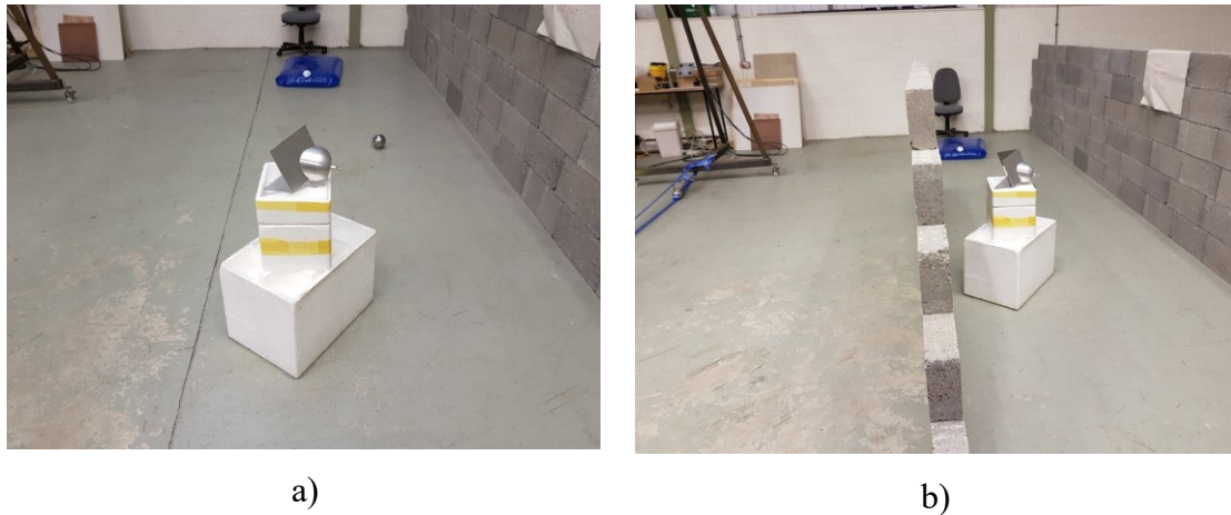
Figure 3-15 – a) unobscured and b) obscured trihedral placed a distance of 2.648m from the antennas. The height of the trihedral is 0.705m.
