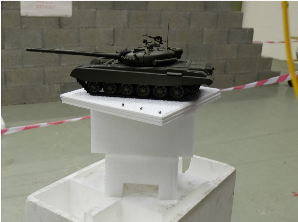
Figure 7-7 – The 20 th scale T72 tank used to illustrate high frequency spatially variant basebanding. The tank is raised on a polystyrene plinth, this is in order to separate the backscatter from unwanted clutter and multipath signatures, and better centre the tank inside the aperture.
