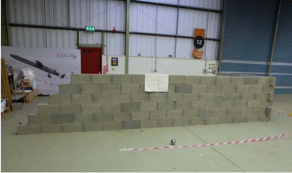
Figure 6-3 – The 1.3m high concrete wall placed 3.6m from the SAR system. In addition to the wall structure, a metal sphere is placed prominently in the scene. This is to aid image coregistration.
