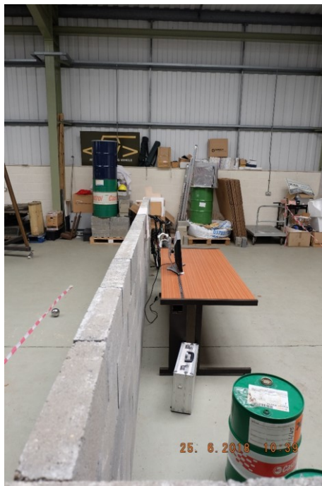
Figure 7-13 – Side on view of the same scene, showing the proximity of each element to the wall. A metal sphere has been added in front of the wall to help calibrate different measurements.
