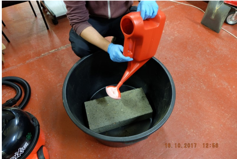
Figure 3-5 – Photograph showing the concrete sample block being soaked with 5% by mass of deionised water.
