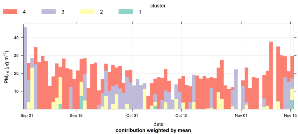
Figure 4-10: Temporal variation in daily PM_{2.5} concentration at UCC by the contribution of each cluster for the entire period of deployment
