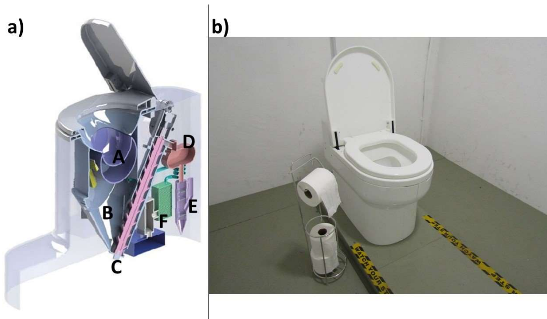
Figure 1-1: NMT. a) schematic drawing of its components: A - mechanical flush, B - collection tank, C - auger, D - dryer, E - combustor, F - membrane bundle; b) photograph of an NMT prototype for field testing.
