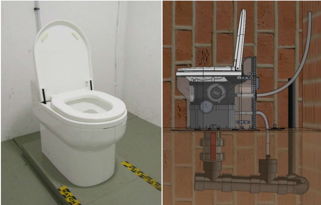
Figure 2-2: a) prototype pedestal with mechanical waterless flush, installed in a dedicated toilet room adjacent to the laboratories of the Pollution Research Group at the University of KwaZulu-Natal; b) schematic of the installation: The pedestal is connected to the sewer mains and has a ventilation pipe from inside the unit. The gear system is shown to be on the side of the pedestal, underneath the cover
