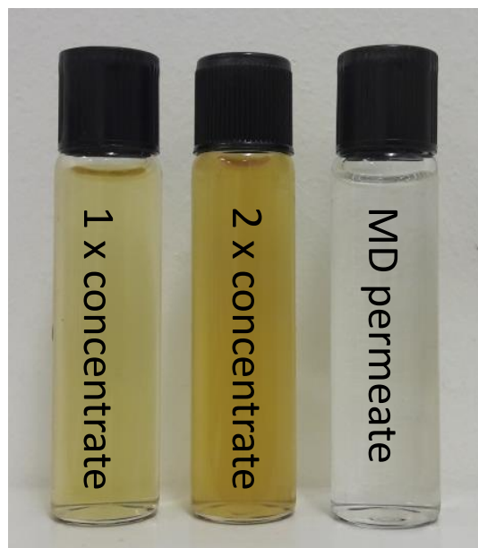
(a) Figure S 5.3 Real urine (1x and 2x concentrated) and membrane distillation (MD) permeate polarisation curves (b) visual comparison of real urine and MD permeate solutions. Real urine concentration was 12.45 \text{ mS cm}^{-1} , 2x concentrate was 24.1 \text{ mS cm}^{-1} , and permeate was \sim 0.2 \text{ mS cm}^{-1} .
