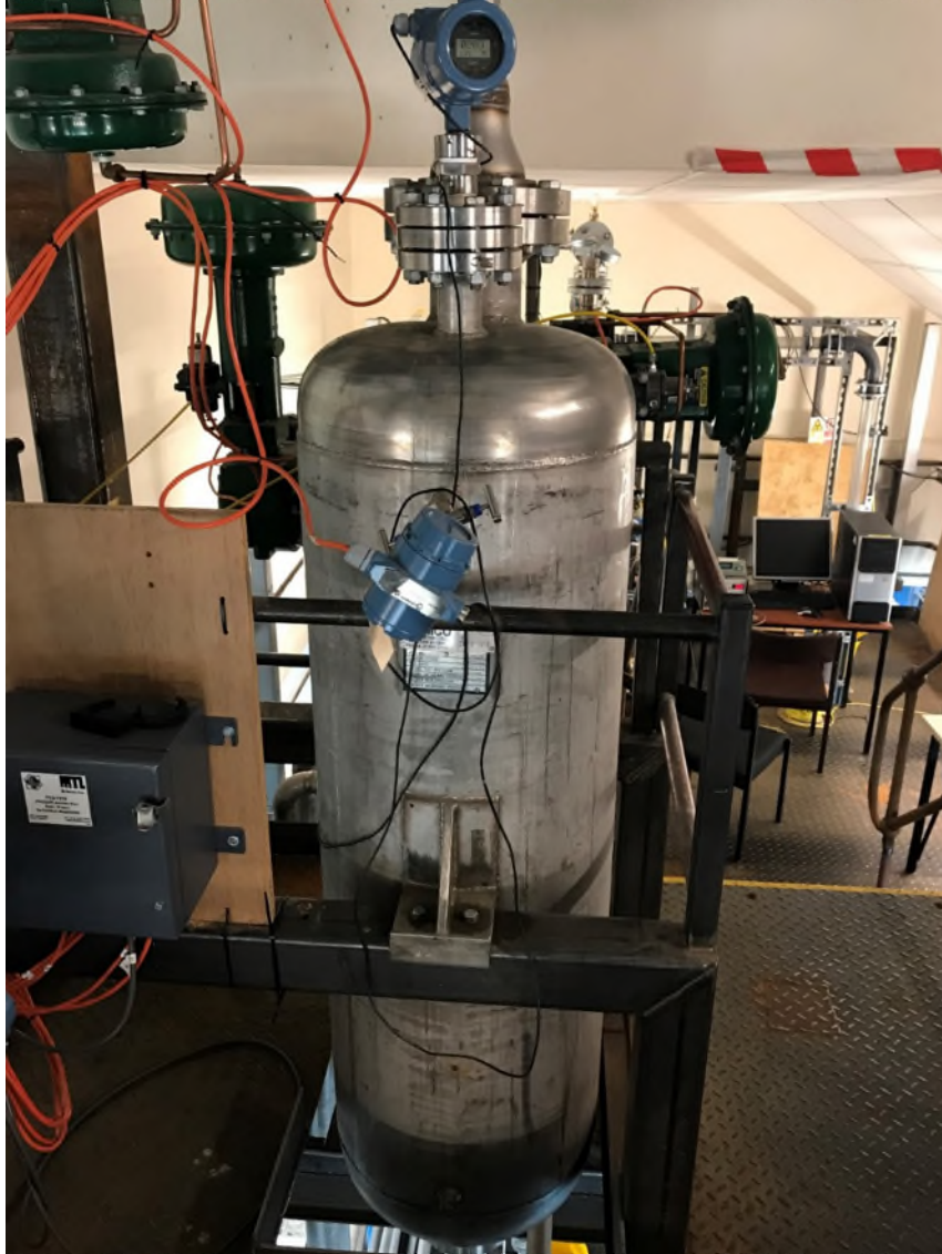
Figure A.4-1 Topside two-phase separator
