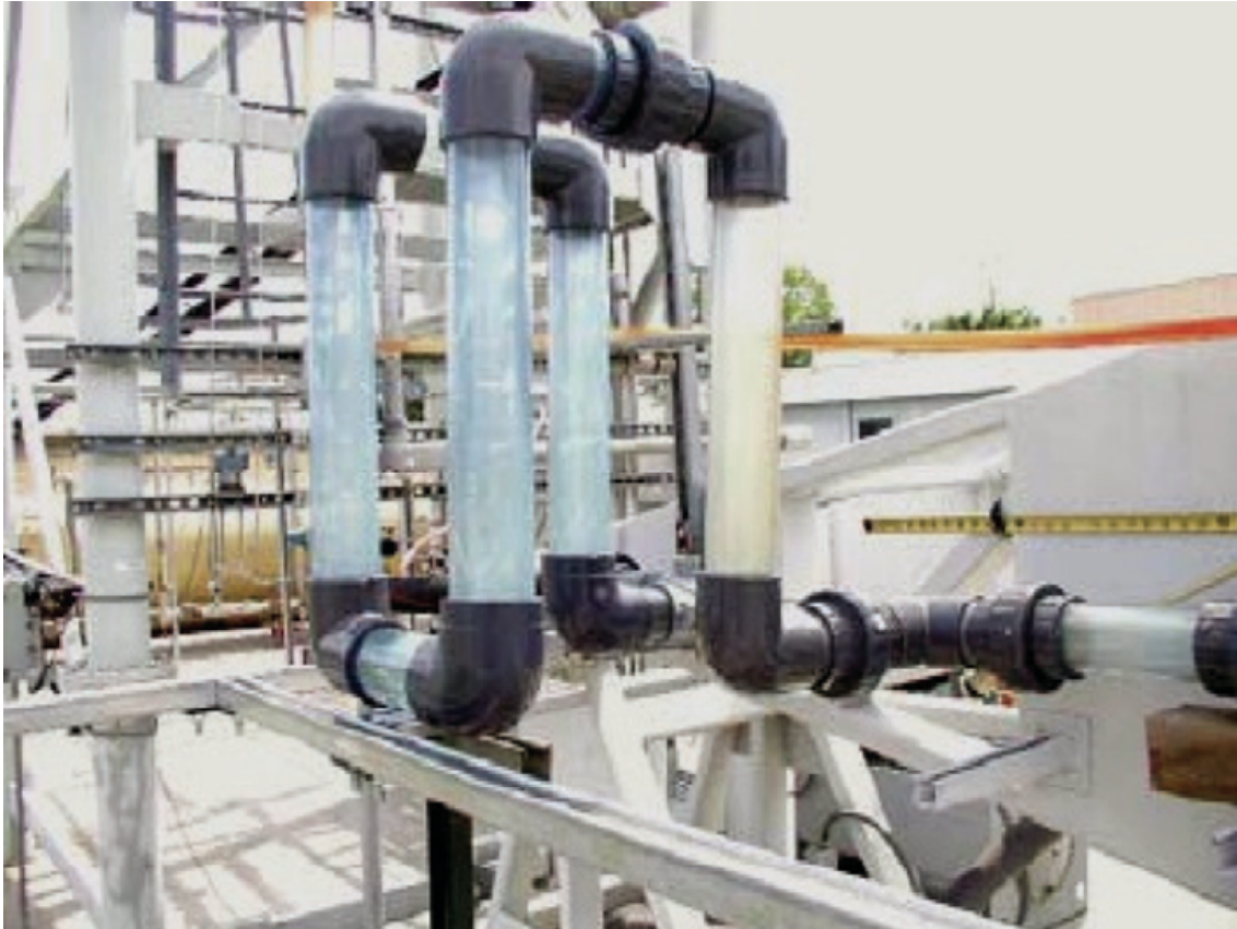
Figure 2-16 Non-intrusive passive device severe slug attenuation device (Makogon et al., 2011)
