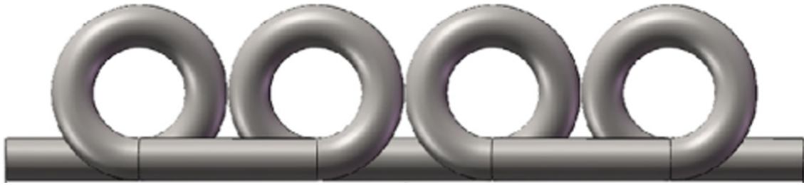
Figure 2-18 Schematic of the quasi-plane helical pipe (Yao et al., 2019)
