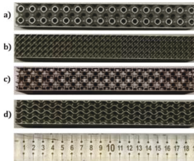
Figure 11. Experimental samples with lattice structures of (a) primitive (b) diamond (c) IWP (d) gyroid (Reproduced with permission from. [105] Copyright 2021, Springer)
