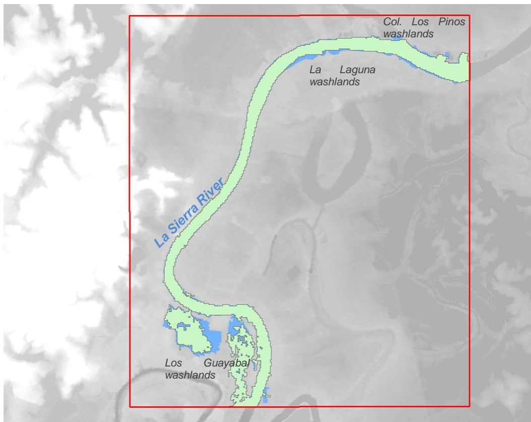
Figure 5.24: The simulated flood extents (light green) and satellite-derived contours (blue) underline the adequate capacity of the calibrated model to replicate the actual observed flooded area.
