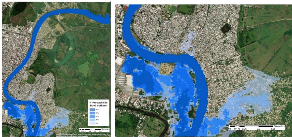
Figure 5.31: Probabilistic flood inundation extent outlines in the 5% and 95% confidence limits based on ensemble model runs based on high Strickler parameter value scenario.
