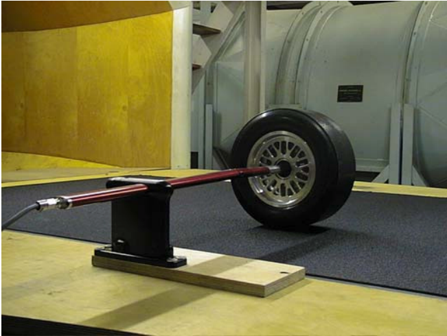
Figure 3: Experimental Set-up showing Parallel Wheel and Support Sting
