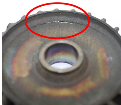
Fig. 11. Additive manufactured turbine wheel failed after hot test
