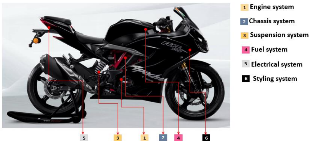
Figure 1-2 Model of two-wheeler and its critical sub-systems [4]
