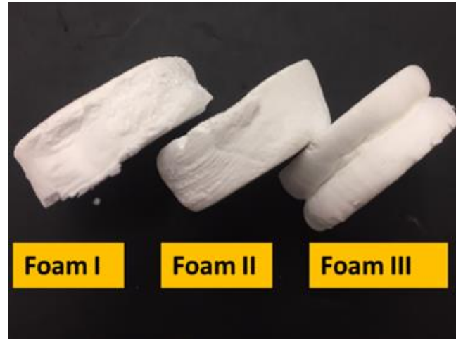
Figure 58: Failure mechanisms observed in PSNF/PVA foams.
