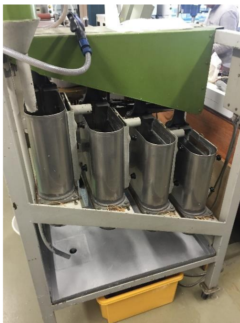
Figure 27: Bauer-McNett classifier for fibre length analysis
