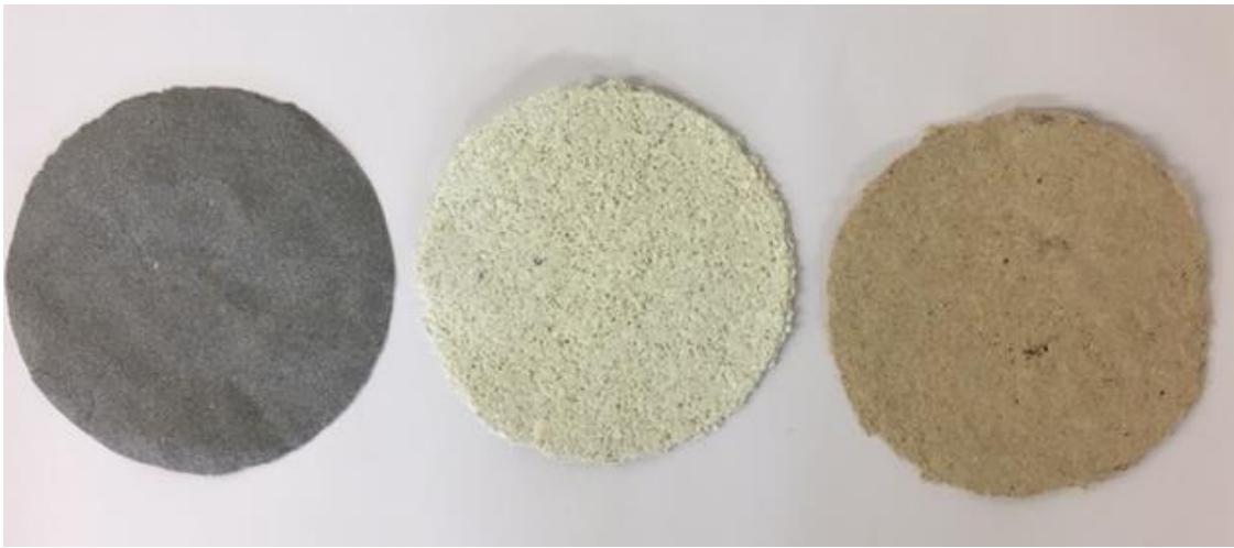
Figure 19: Hand sheets prepared from different PMS (L to R: JCR, TPK and UPH).
