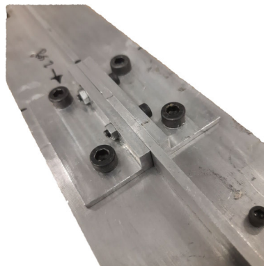
Figure 7.3: XB-2: Reinforcement plates of the wing spar.
