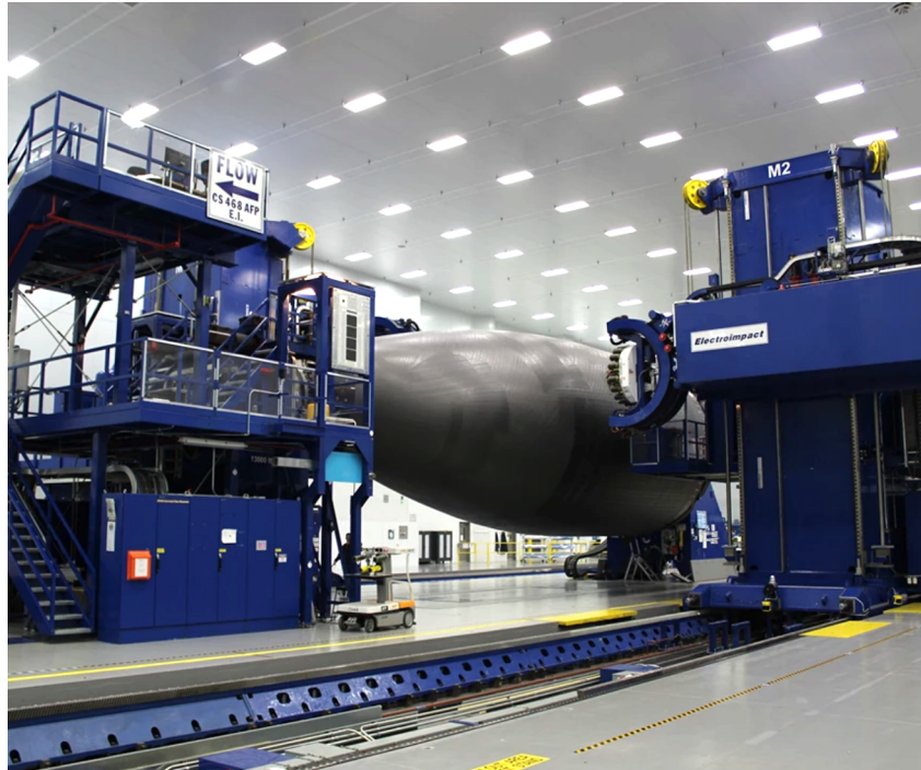
Figure 1.2 Manufacture of monolithic fuselage section for the 787 Dreamliner with AFP on a rotating mandrel. Reproduced with permission from CompositesWorld [9].
