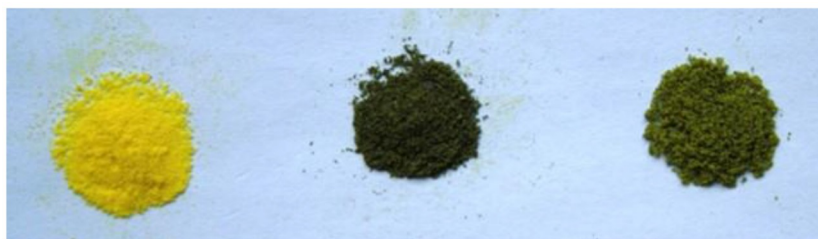
FIGURE 10 Photos (from left to right) of pure FOX-7 and its mixtures with CTAB and Citrate capped GNPs at 2 wt.% concentration, respectively.
