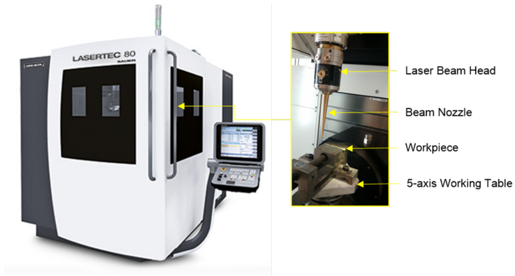
Figure 3-3. Laser machine used for the drilling of the samples.
