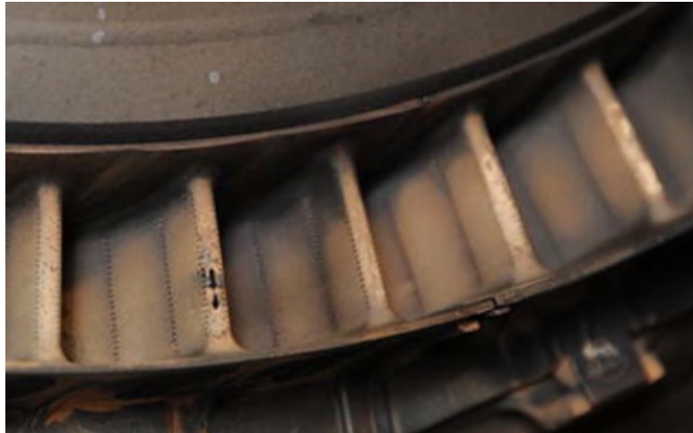
Figure 2-3. Photograph of thermal cracking and overheating in nozzle guide vanes (Mishra, Johney, et al. , 2014).
