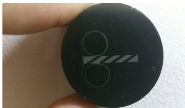
Figure 3-7. Resin mounted laser drilled sample for metallography examination.
