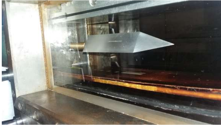
Fig. 4 Pyramidal model mounted on the sting strain-gauge balance in the test section
