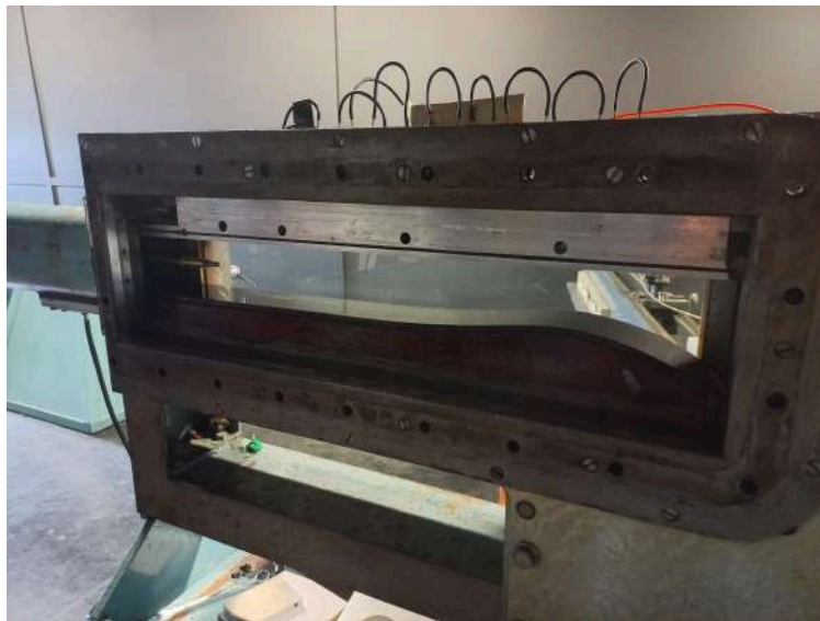
Fig. 5 Wind Tunnel Working Section without a model and the Mach 1.6 Supersonic Liner
