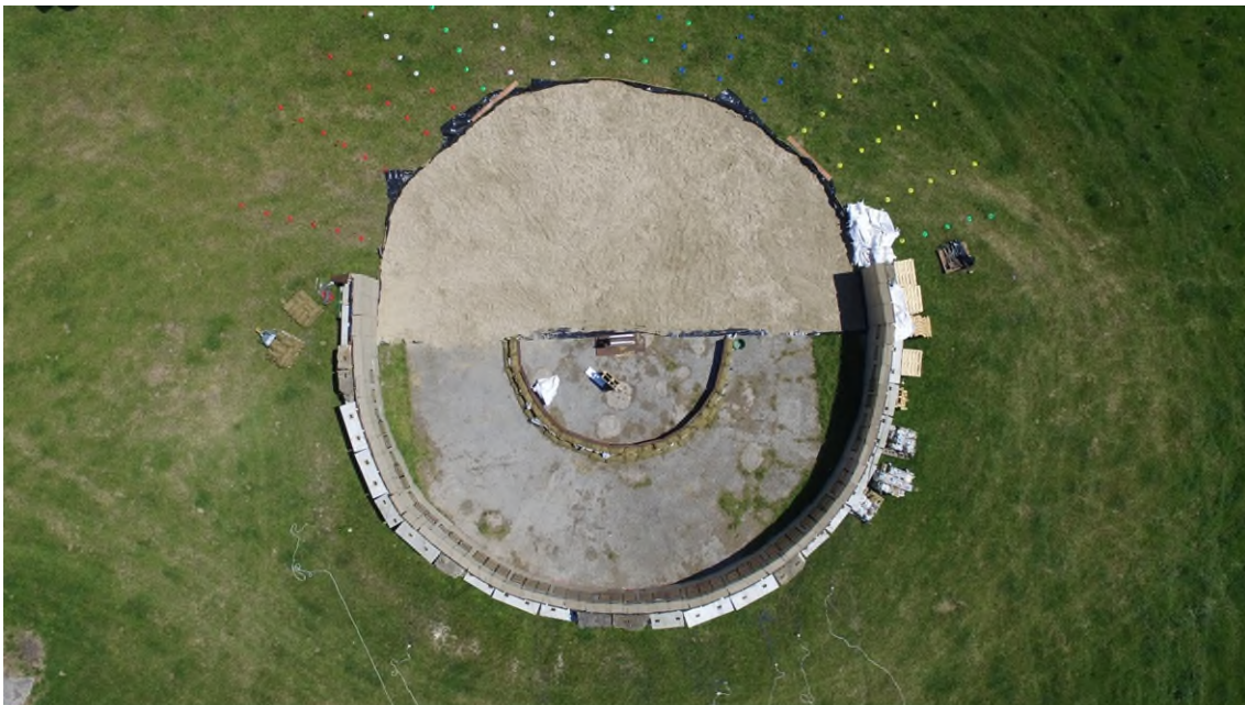
Figure B.1 2 – Arena completed with the sand for the environmental collection and the fragment arena for fragments collection
