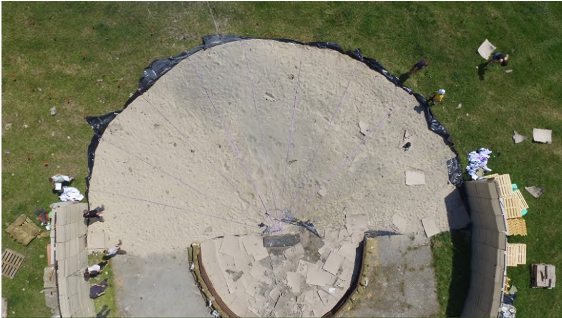
Figure B.2 1 - Post-detonation residues after detonation 1 with munition in horizontal position
