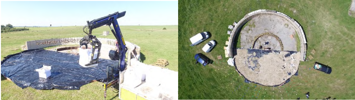
Figure B.1 1– Arena set up. On the left the black plastic groundsheet to avoid cross-contamination from the soil underneath. On the right the laying out of the sand.
