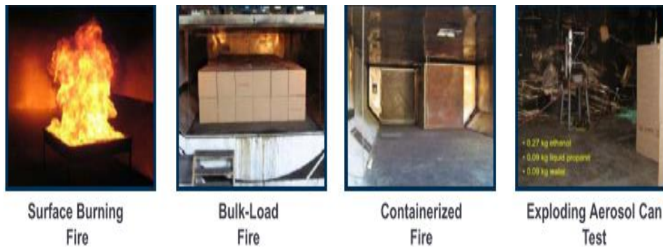
Figure 119 - MPS fire test scenarios for aircraft cargo [3]
