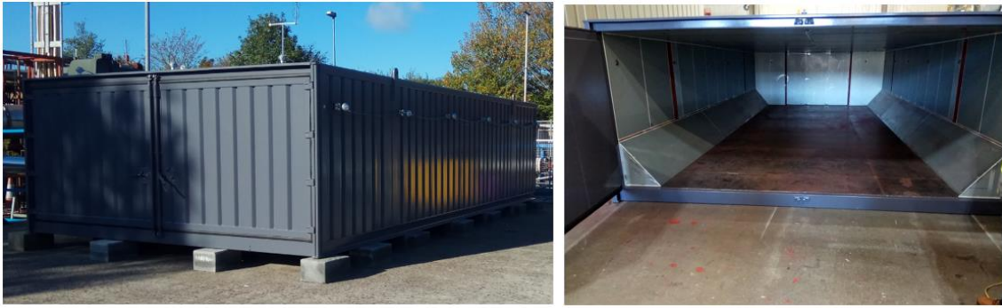
Figure 103 - Test rig cargo compartment structure
