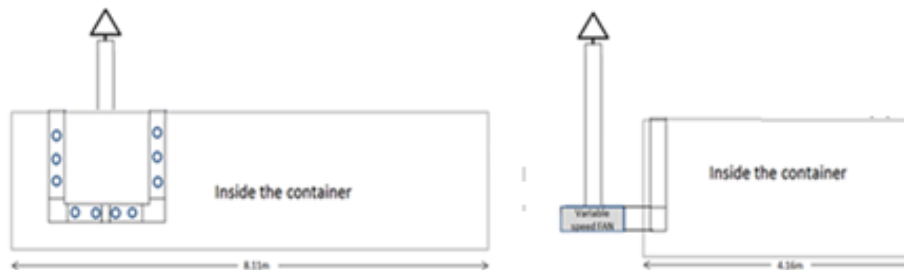
Figure 32 - Test rig ventilation system arrangement for Halon1301 (FAA)
