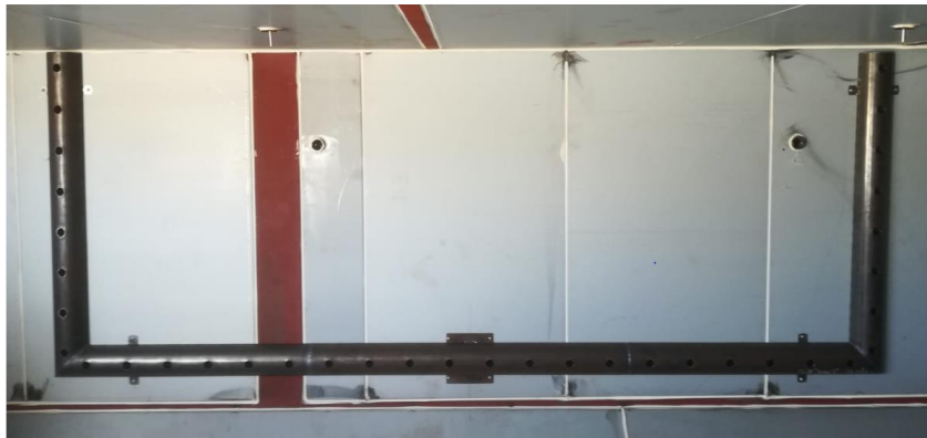
Figure 104 - Cargo door leakage representation on test rig
