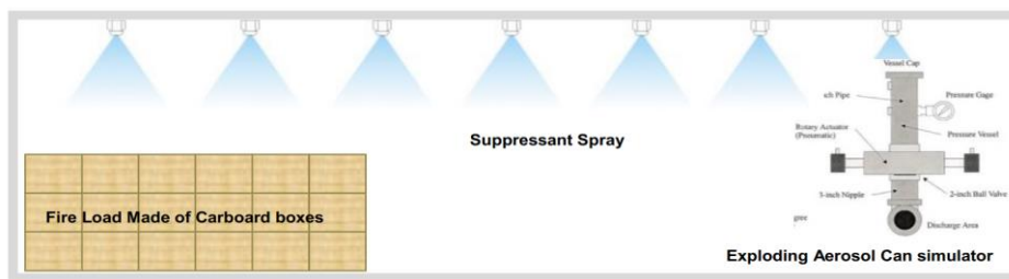
Figure 129 - Aerosol can explosion test
