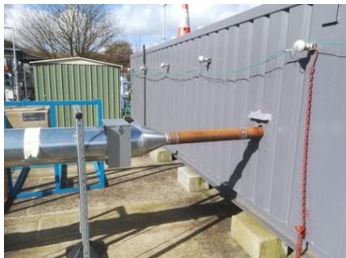
Figure 105 - Variable speed fan connected for cargo door leakages
