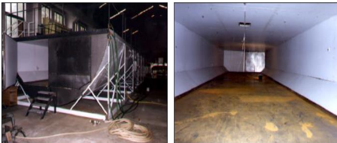
Figure 22 - Experimental test rig of FIREDASS for MPS tests using water mist [77]
