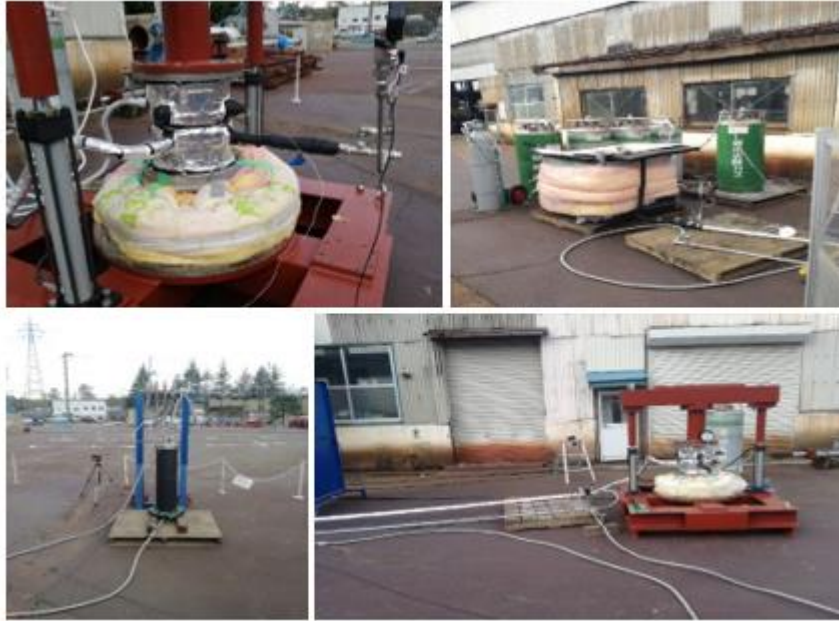
Figure 5-5: Pictures of the experimental apparatus - left-to-right and top-to-bottom: vessel coupler; methanol-nitrogen refrigeration; buffer container; inlet, outlet pipework and pressurised oil system
