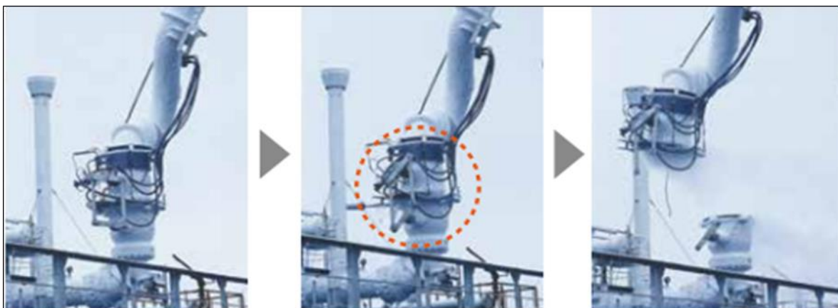
Figure 5-1: Sequence of the operation of ERS; 1) separation begins; 2) the two valves shut completely; 3) Emergency Release Coupler opens completing the separation [14].
