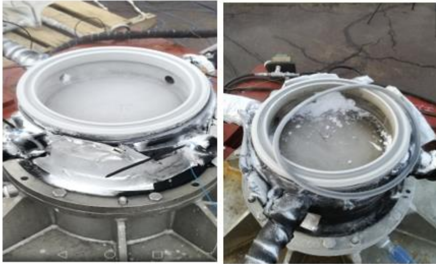
Figure 5-11: Bottom surface of the test vessel after the experiment; Test 2.1 (left), Test 1.1 (right)
