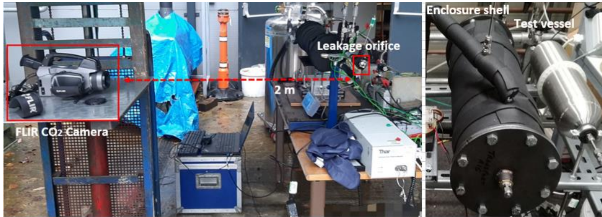
Figure 4-3 : left-to-right CO 2 camera acquisition view; enclosure shell and test vessel prior to assembly
