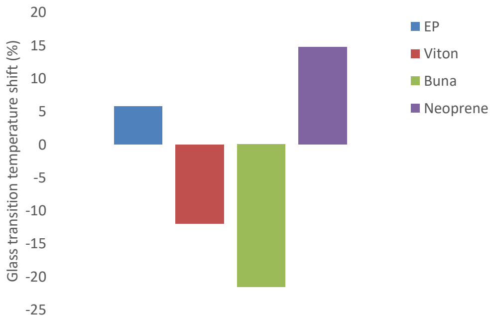
Figure 3-11: Summary of average % glass transition shift of materials under CO 2 pipeline tests
