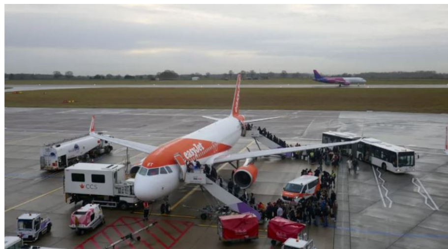
Figure 2. Ground support equipment and vehicles servicing aircraft.
