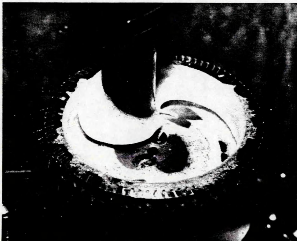
Plate 2 Problem of foaming with surfactant
