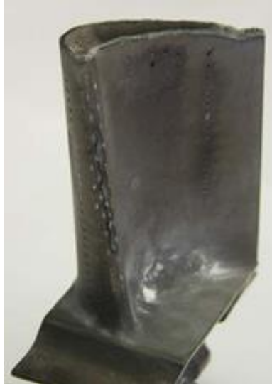
Figure 2-6 Leading edge erosion
