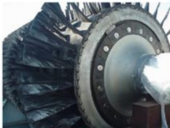
Figure 2-2 Oil deposits on axial compressor blades [29]
