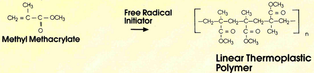
Figure 4.1 Basic chemical structure of Modar 8035 and the resin network.
