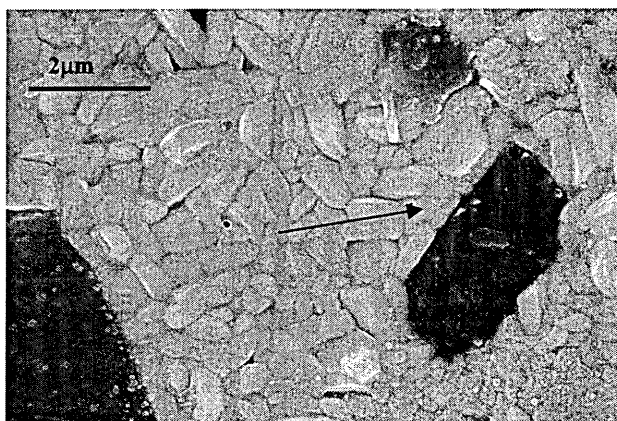
Figure 3.74: Final stage of the formation of big magnesium titanate grains due to the evaporation of bismuth. The arrow indicates the completely formed \text{MgTiO}_3 second phase.
