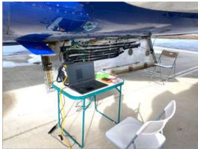
Figure 4 Ground test facility of the Boeing 737-400, Left-side PACK data collection
