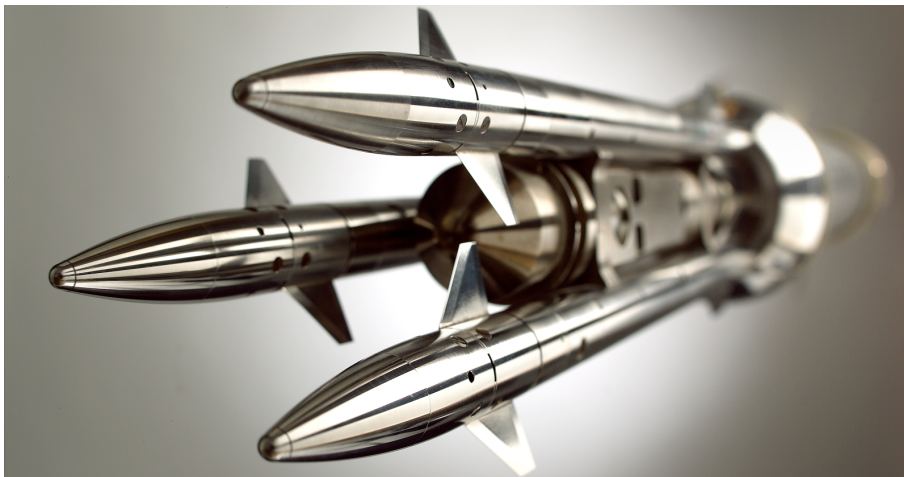
FIGURE 1.0.7 STARSTREAK dart submunitions mounted on main rocket body [21]
