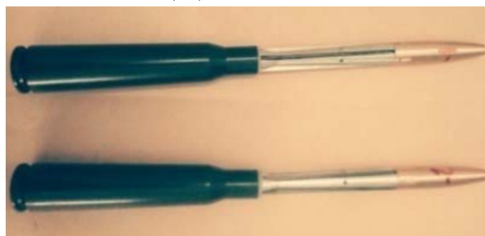
(B) Prototype in cartridge without sabot
