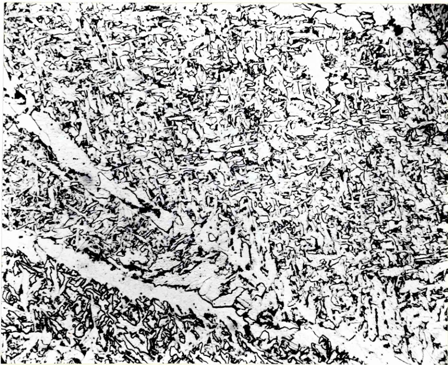
Figure 87 Weld 850 amp - 300 mm/min. Sub-Surface as deposited structure x 500
