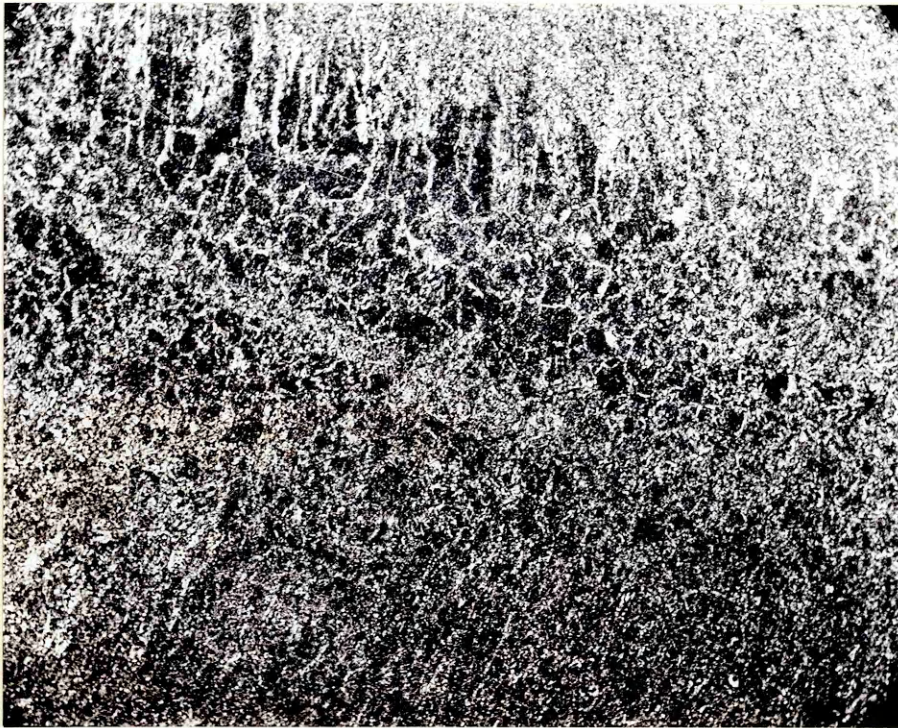
Figure 103 Weld 480 amp - 300 mm/min. Root Columnar Structure x 50
