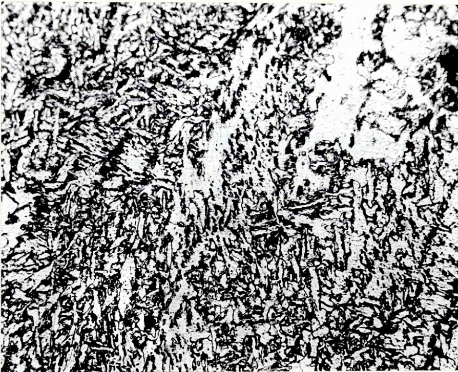
Figure 105 Weld 480 amp - 300 mm/min. Root as deposited structure x 500
