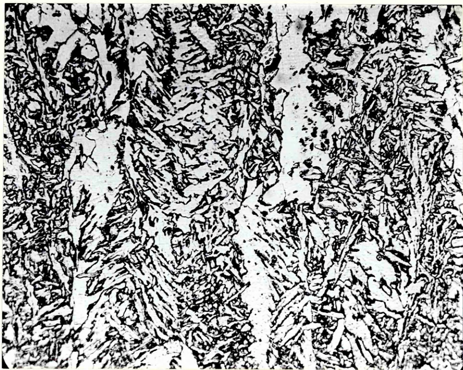
Figure 57 Weld 650 amp - 200 mm/min. Root as deposited structure x 500
