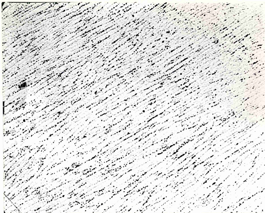
Figure 72 Weld 650 amp - 400 mm/min. Sub-Surface ↳ Ferrite Structure x 50
