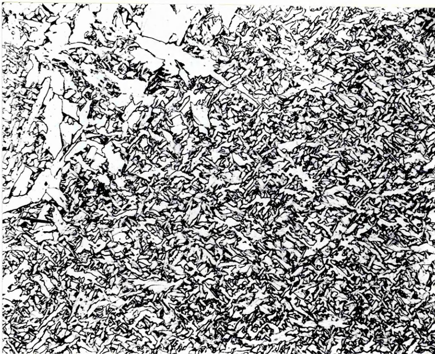
Figure 99 Weld 480 amp - 300 mm/min. Sub-Surface as deposited structure x 500
