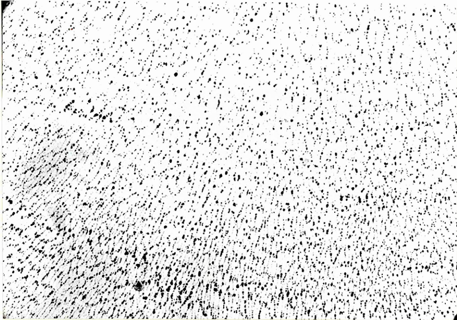
Figure 54 Weld 650 amp - 200 mm/min. Root \delta Ferrite Structure x 50
