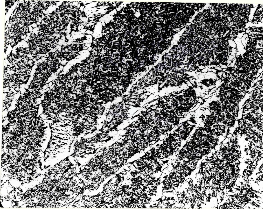
Figure 62 Weld 650 amp - 300 mm/min. Sub-Surface as deposited structure x 200
