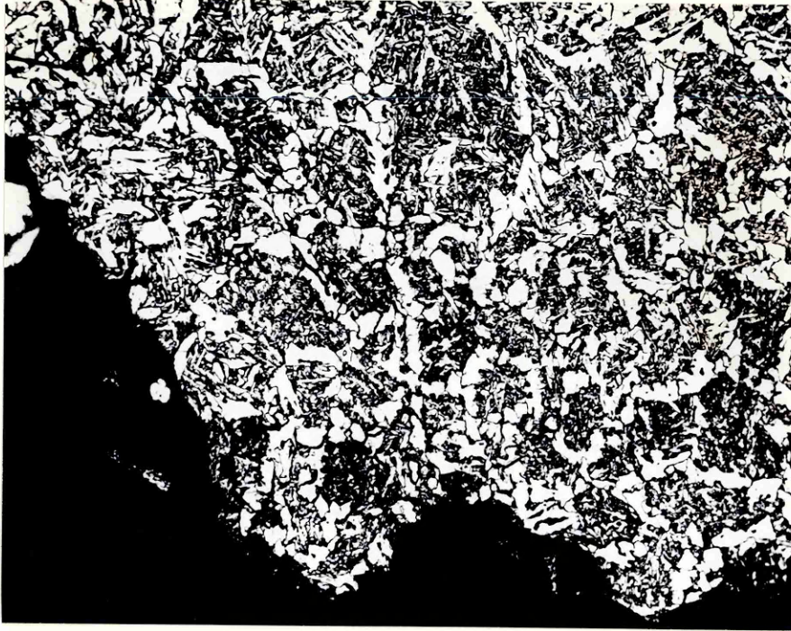
Figure 94 Weld 850 amp - 300 mm/min. Root Charpy V fracture path x 200
