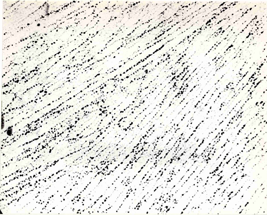
Figure 84 Weld 850 amp - 300 mm/min. Sub-Surface Ferrite Structure x 50
