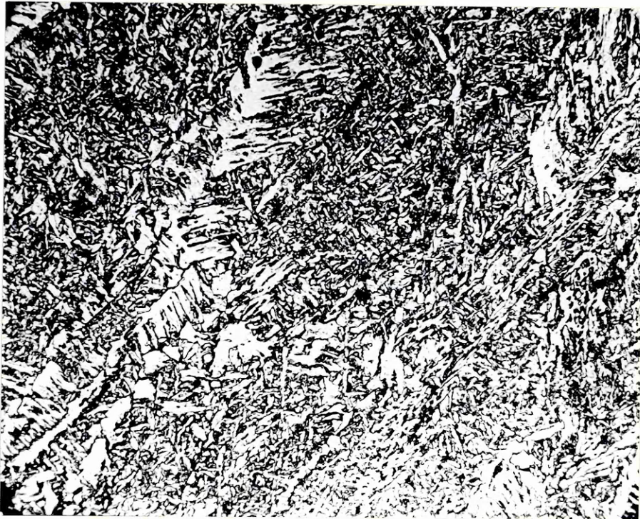
Figure 81 Weld 650 amp - 400 mm/min. Root as deposited structure x 500
