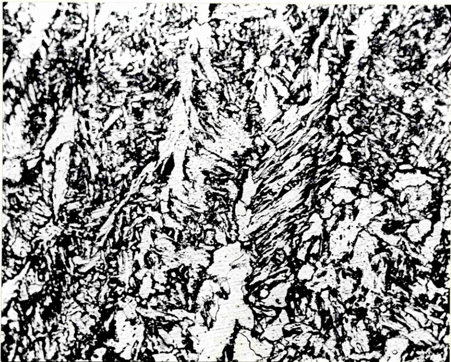
Figure 69 Weld 650 amp - 300 mm/min. Root as deposited structure x 500
