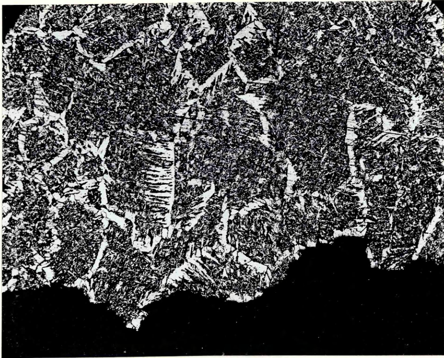
Figure 52 Weld 650 amp - 200 mm/min. Sub-Surface Charpy V fracture path x 200
