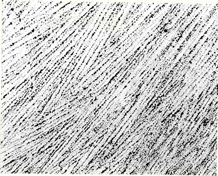
Figure 60 Weld 650 amp - 300 mm/min. Sub-Surface δ Ferrite Structure x 50
