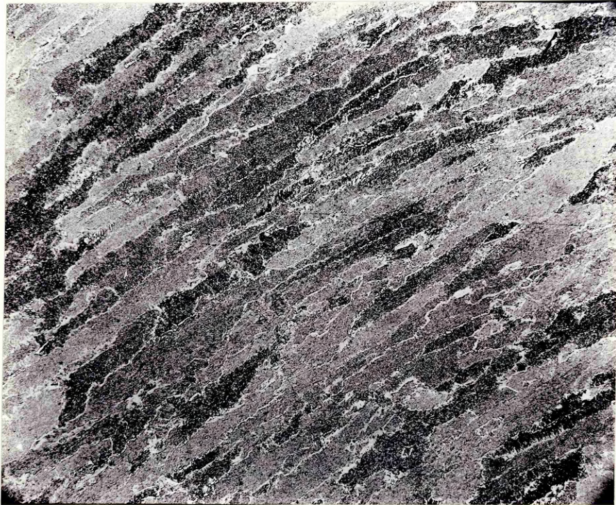
Figure 61 Weld 650 amp - 300 mm/min. Sub-Surface Columnar Structure x 50
