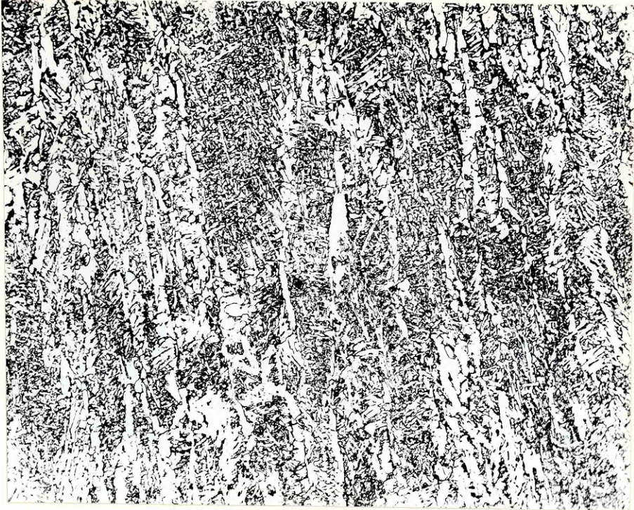
Figure 56 Weld 650 amp - 200 mm/min. Root as deposited structure x 200
