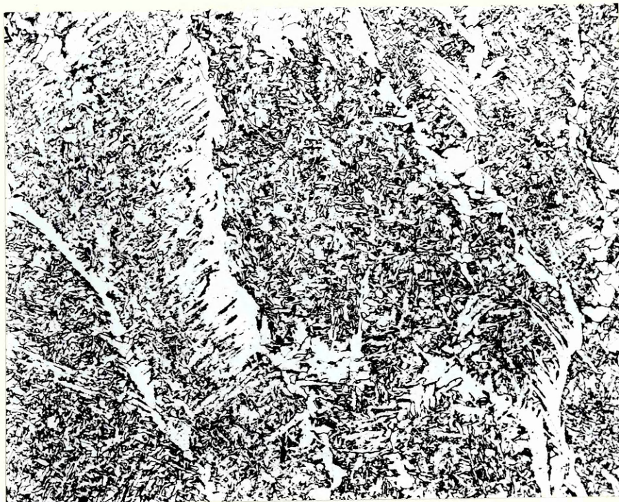
Figure 50 Weld 650 amp - 200 mm/min. Sub-Surface as deposited structure x 200
