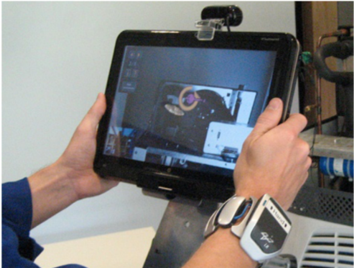
Figure 2.12. Example from Webel [30] of the utilisation of vibrotactile bracelet (on the right arm) for supporting maintenance task. Tabled with external camera pointing and the object to maintain. The AR animation is displayed on the tablet screen.
