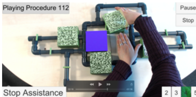
(e) Real object becomes green when aligned with virtual object suggested position.
