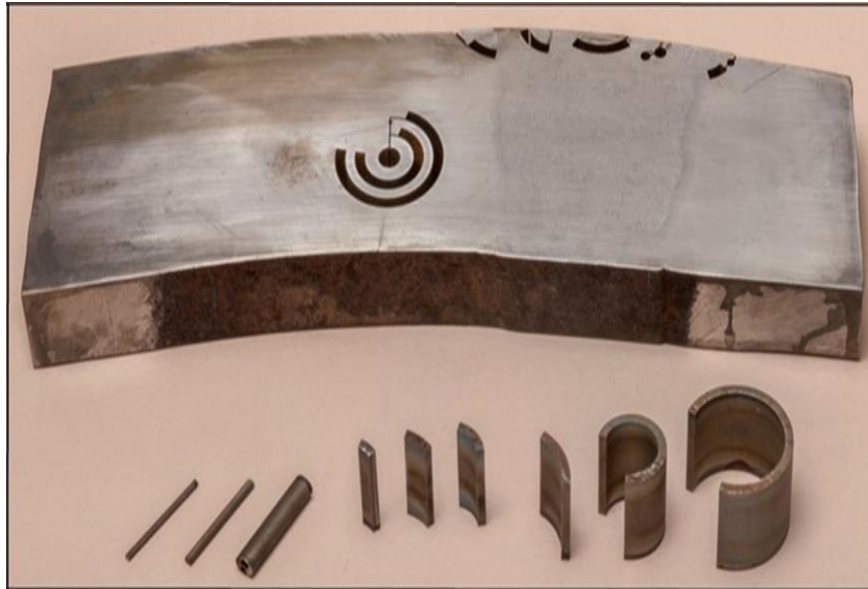
Figure 3-3 The cut pieces of metal from the weldment after electrical discharge machining (EDM)
